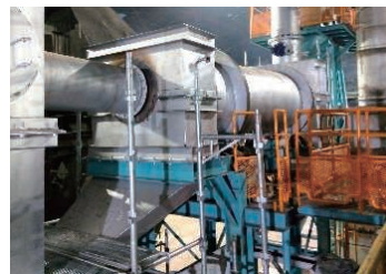
Installation of material preheating equipment (to remove moisture and oil)
