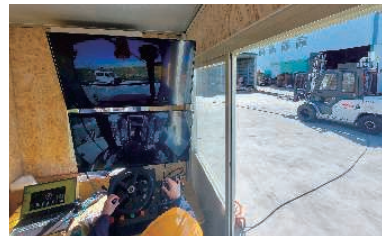
Remote operation of forklifts
