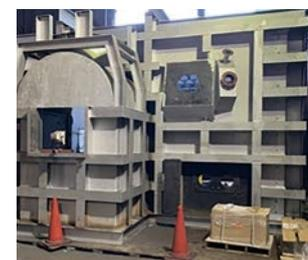
Photo 2: Heat insulation paint
