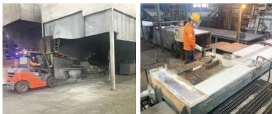
We remelt aluminium scrap and adjust its components optimally in accordance with customer needs. It is then recycled into aluminium alloy ingots through refining and casting processes. In our alloy business, in addition to supplying ingot products, we supply molten aluminium alloy that does not require remelting, and we manufacture environmentally friendly products in our horizontal recycling (including can-to-can recycling) and other businesses.
