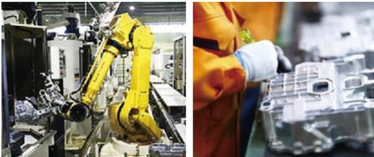
Using recycled aluminium ingots and molten aluminium alloy produced within the Group, we cast, process, and assemble die-cast parts mainly for automobiles. Our mass-productivity, high-quality die-cast products have a wide range of applications, including automobiles, two-wheeled vehicles, industrial machines, medical machines, and daily necessities.
