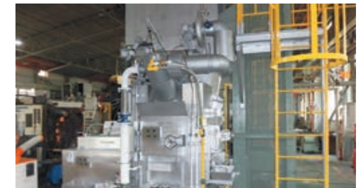
連続溶解保持炉SEH (浸漬型) Continuous melting and holding furnace SEH (immersion type)
